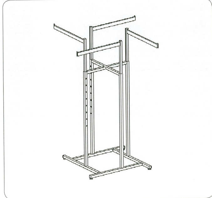
#0506 Base of 1" square tubing with 4 adjustable levellers. Four 22" straight arms of 1/2" x 1 1/2" rectangular tubing.
